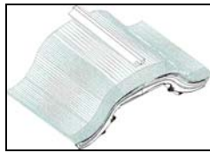
Figure 10b: Entrance canopy – wire frame CAD model
