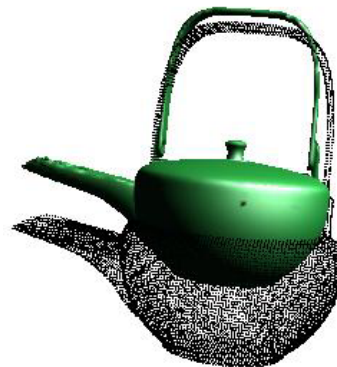
Figure 13: Point data set used for reverse construction (black) and an intermediate shape during the fitting process (green).
