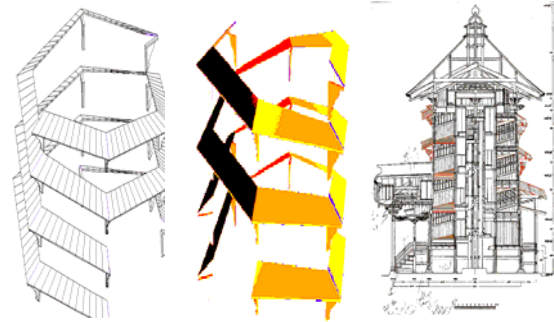
Figure 5: Exterior tower overhang: (L) wire frame; (M) colorized; (R) diagram of the exterior overhang location.
